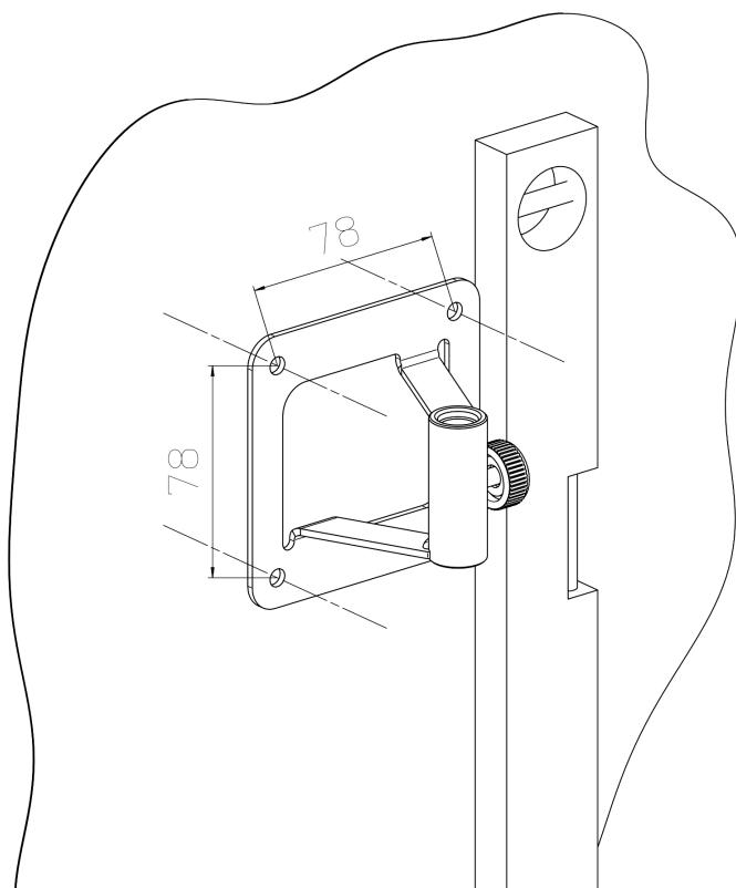
All four holes of the wall bracket must be used for fastening. A suitable fastener must be selected according to the wall condition.
