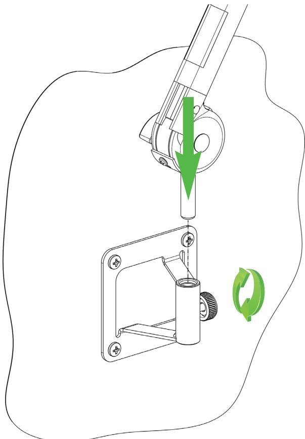
Loosen the clamping screw on the wall mount. Insert the microphone desk arm into the wall mount from above, adjust to the desired position and hand-tighten the clamping screw.
