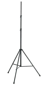
This compact overhead microphone stand is now even lighter and more stable. Thanks to a new leg combination and a new clamping element, its weight has been reduced to 3.8 kg. The leg base diameter of 1 m affords stability and safety. A range of different boom arms can be attached using the 3/8" thread adaptor. The stand extends to a height of over 3 m.
