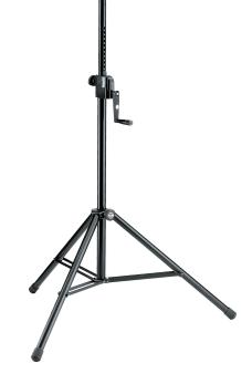
A high quality steel speaker stand with zinc die-cast clamps for professional use. Infinitely variable height adjustment with a hand crank and push button system which prevents an uncontrolled reverse motion. There is an additional locking screw for extra safety. Extension tube diameter 35 mm, suitable for speakers and lighting crossbars with an integrated M10 thread connector.
