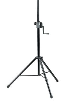
A high quality steel speaker stand with plastic clamps for professional use. Infinitely variable height adjustment with a hand crank and push button system which prevents an uncontrolled reverse motion. There is an additional locking screw for extra safety. Extension tube diameter 35 mm, suitable for speakers and lighting crossbars with an integrated M10 thread connector.
