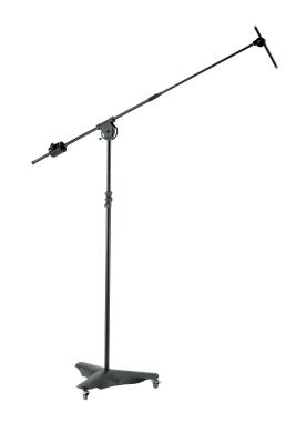
Mobile heavy steel microphone stand for studio or stage. 10 kg cast metal base, low centre of gravity for high level safety with 3 lockable castor wheels. Rod combination extends to over 2 m with additional locking mechanism. Extendable boom arm with a 3 kg counterweight and 5/8" connecting thread. Additional mini boom arm with 5/8"- and 3/8"- connecting thread, fully adjustable regardless of the position of the main boom arm, e.g. to use with studio microphones.
