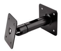
The practical wall and ceiling mount for smaller loudspeakers has been upgraded. A new feature is a cable outlet, which now provides an internal cable guide for hidden installations. Thanks to two special threaded pins and the Allen wrench / hexagon key included in the delivery, the universal joint can be positioned and set exactly. As such the load capacity increases to 10 kg. The wall distance has been reduced to 160 mm.
