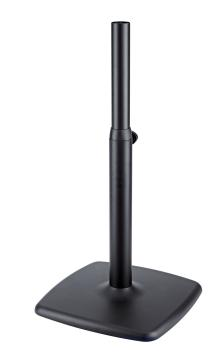
Impressive steel stand for monitors with stable, elegant cast base 480 x 480 mm. The large-dimensioned tube combination is gradually height adjustable by means of a spring-loaded clamping knob from 644 to 1044 mm. Depending on the size of the monitor, three different bearing plates 26792 can be mounted.
