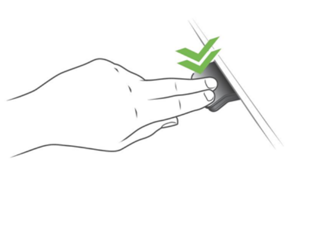
Figure 3: Press twice to move the keyboard table automatically to a prestored position.
