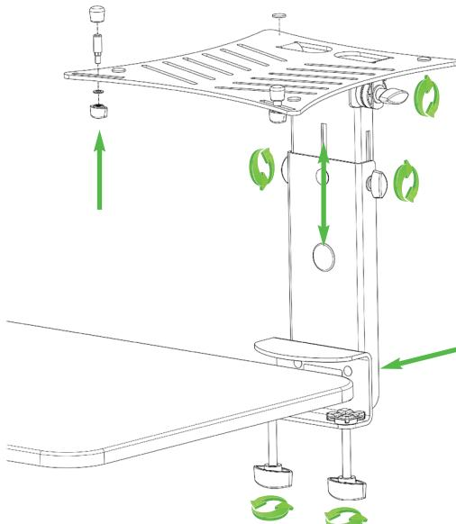
Open the clamping screws on the table clamp until the table clamp can be slid over the tabletop. Make sure that the table clamp rests completely against the edge of the table. Tighten the clamping screws hand-tight.
