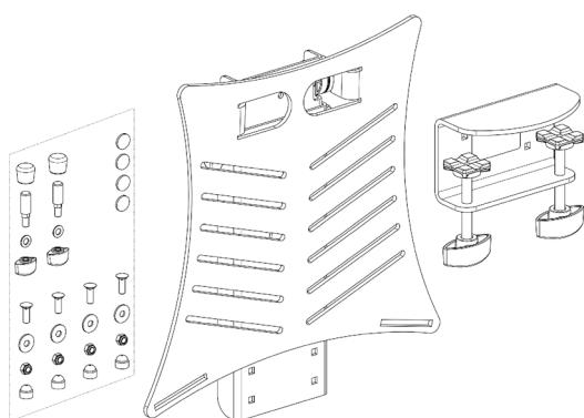
Accessory bag: 2x protective cap, 2x stop pins, 2x washer ø10 mm, 4x Clamping nut
