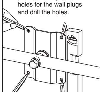
Hold the wall plate in place vertically, mark the holes for the wall plugs and drill the holes.
