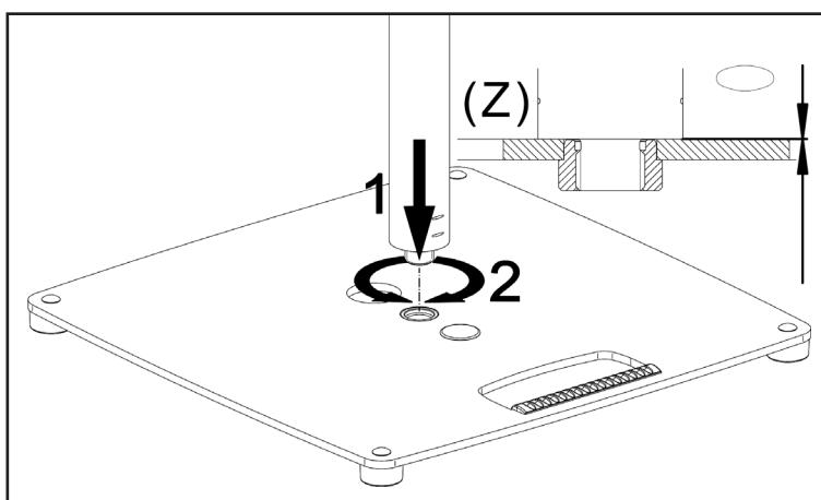
Place the distance rod to be fitted on the base plate **1**, and screw it completely into the base plate **2**.
