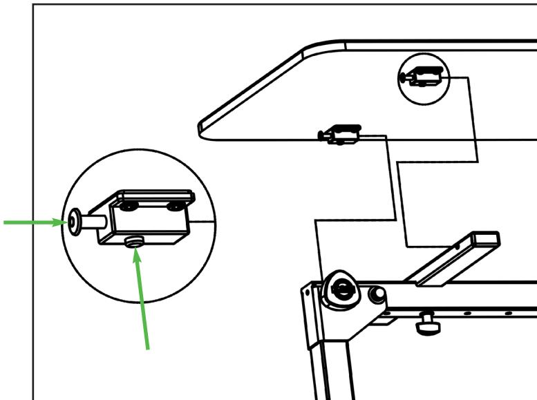
To rest the tabletop on, the four safety catches must be "opened". To do this, press the red button on the catch. The locking pin snaps back and the tabletop can be mounted.
