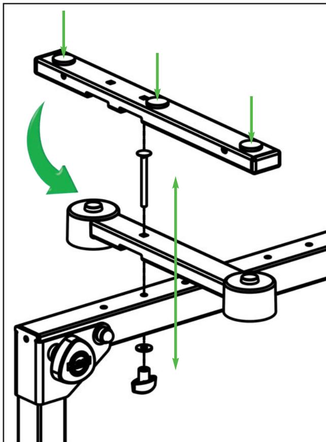
To mount the tabletop, the support tubes of the »Omega« must be exchanged for the support tubes of the tabletop. To do this, loosen the clamping nut and remove it together with the washer. Remove the support tube upwards from the »Omega«. The support tubes of the tabletop are mounted in reverse order. Make sure that one bore at the outside remains free and that the long side of the support tubes points to the long side of the foot tubes, see note.
