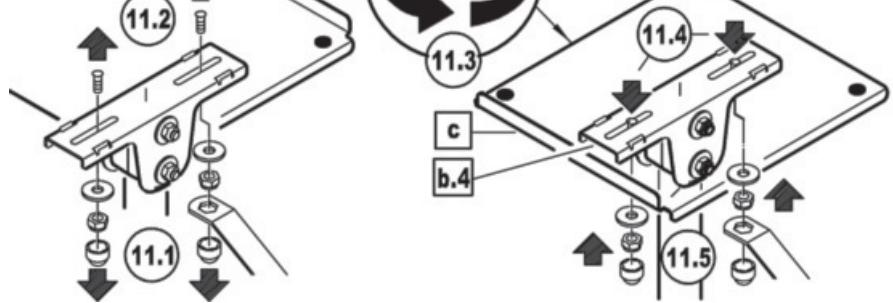
**12. CENTER the WEIGHT BEARING LOAD by ADJUSTING the TRAY**
