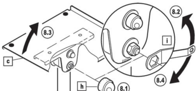
NOTE: Carefully place the monitor on the tray and check to see if the tray moves. If yes, tighten the screws.
