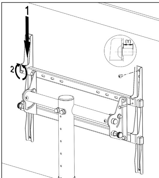
Place the screen on a flat, soft and clean surface with the display side facing down. For mounting on the stand, the pedestal on the screen (if present) must be removed. Secure the two screen holding fixtures to the screen with screws. Ensure the correct screw length **Y**. This can be found in the operating instructions/installation instructions for the screen used or can be obtained from the manufacturer. The screen holding fixtures must be firmly secured to the screen with two screws each.
