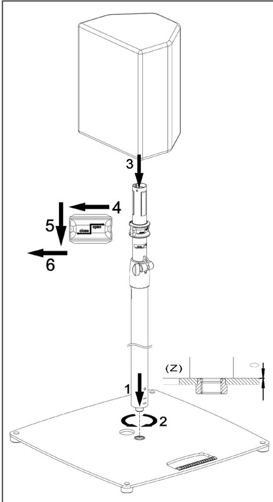
2.) Mount the tube combination on the base
