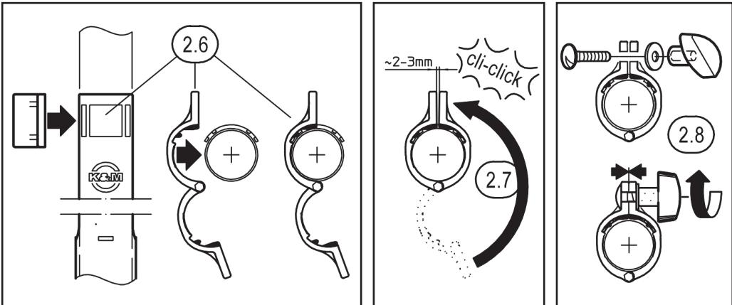
2.7 Now place the other side of the clamping bracket around the leg until it clicks into place, so that there are only a few millimeters between the screw holes.
